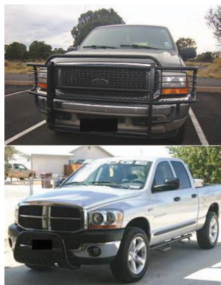
Figure 1 Pickup trucks fitted with a metal bull bar (top) and a nudge bar (bottom) (color figure available online).
